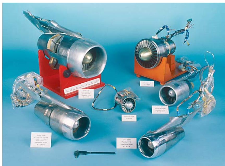
Engine models with Turbine Powered Simulators (M920291)
