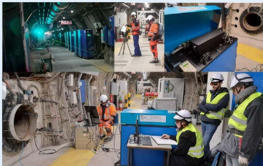
Top left to right: alignment of the emission/reception system with the green pointer, beam deflection mirror and lidar positioned to fire into the cell. Bottom: ONERA-Andra teams.
