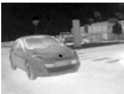
First infrared image with a microbolometer with a pixel pitch of 8.5 \mu\text{m} (QVGA (320x240pixels), optics with a focal length of 3.9 mm open at F/1.2).
