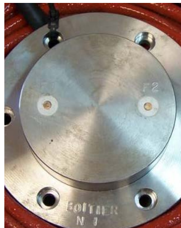
Heat flow measurement block on the VULCAIN 2.1 engine before shipment.
