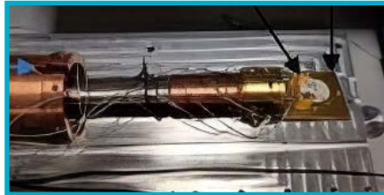
Characterisation of an SHM sensor in a liquid He cryostat environment
