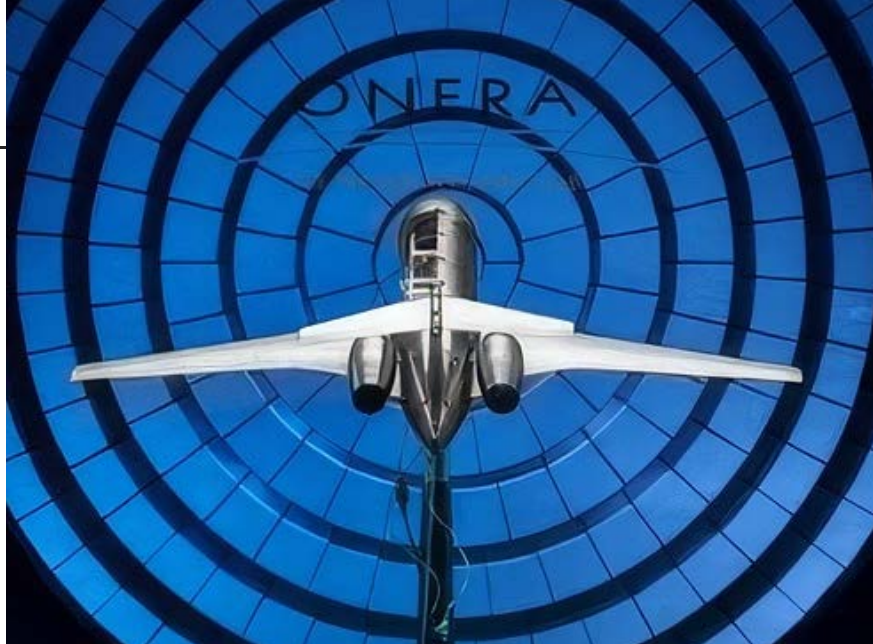
Vein reference configuration. Flow speed: 60 m/s.
