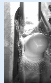
Vein reference configuration. Flow speed: 60 m/s.
