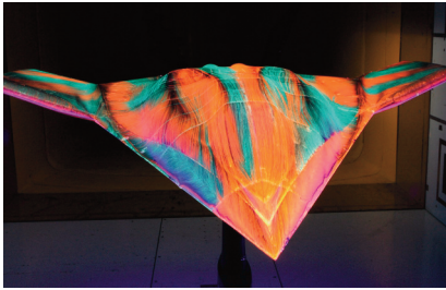
Visualization of the flow over the surface of the Neuron drone (ONERA's F1 wind tunnel)
